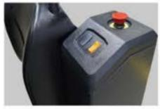
The coasting button on both sides of the truck and emergency stop button allow the operator to operate truck forward/backward while walking beside. There is no need to get in and out of the truck frequently to operate it.At the same time, it reduces the speed while driving forward/backwards under coasting mode, making the traction safer and more efficient.
