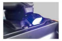
The standard blue light is not only automatically activated when the truck is driving forward, but also turns simutaneously with the handle while steering, which will incrase the safety of operation.
