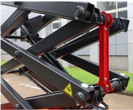
Safety maintenance support bar ensures safety during maintenance.
