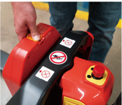
Smart battery positioning and lock for great fixation and safety.
