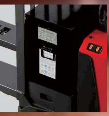
13.8" US tailored open battery compartment ready for wide range of industrial batteries, flexible for different battery dimensions.
