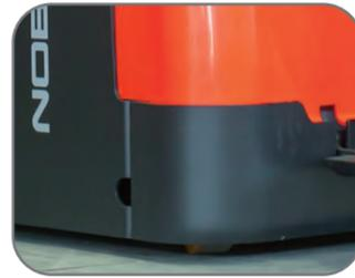
Heavy steel apron provides protection against impact. Steel battery cover provides protection for the battery as well as adding rigidity to the PT55N.
