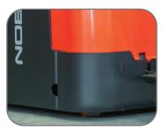
Heavy steel apron provides protection against impact. Steel battery cover provides protection for the battery as well as adding rigidity to the PT55N.
