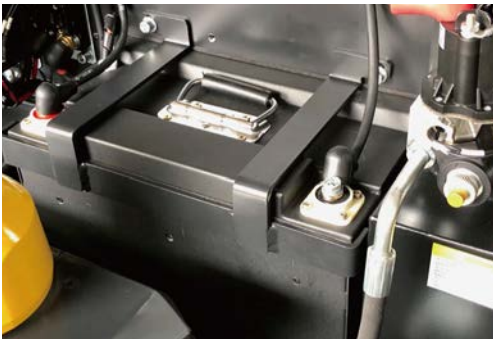
24V/80Ah Lithium-iron battery has connection terminals with screws and is protected inside the steel case.
